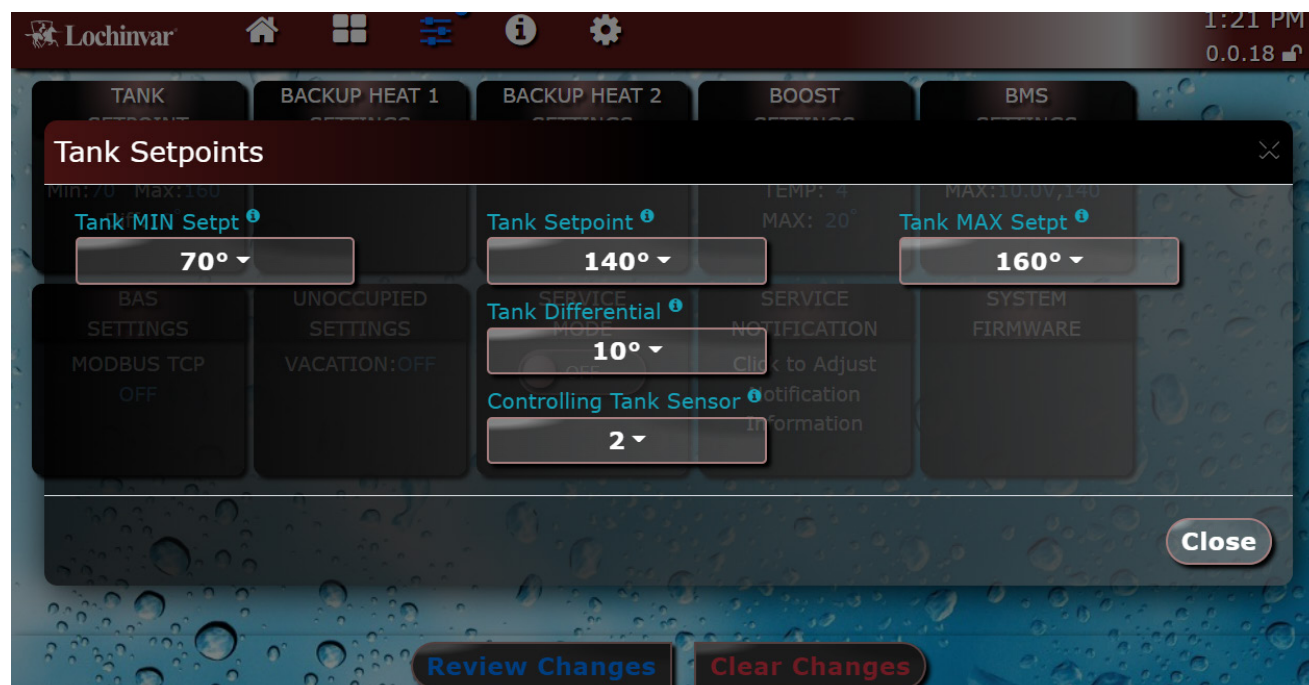
Figure 1-3 Tank Setpoints HW Screen
